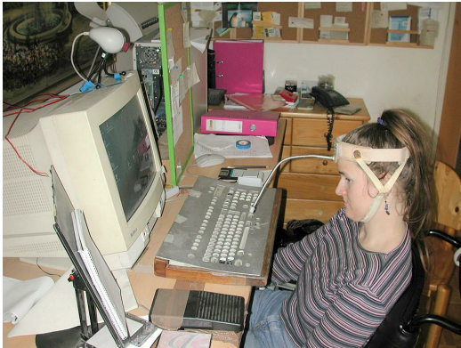
Fig. 5: Non-speaking user of AAC and ECS system [5] using the remote service provision system RESORT over a 64 kbps ISDN link to the university network. This real-life test started at the end of year 2000 and is still on-going using the latest RESORT software version which can be downloaded from [8].
