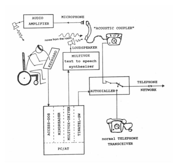
Fig. 1, Components of the TINATEL system
