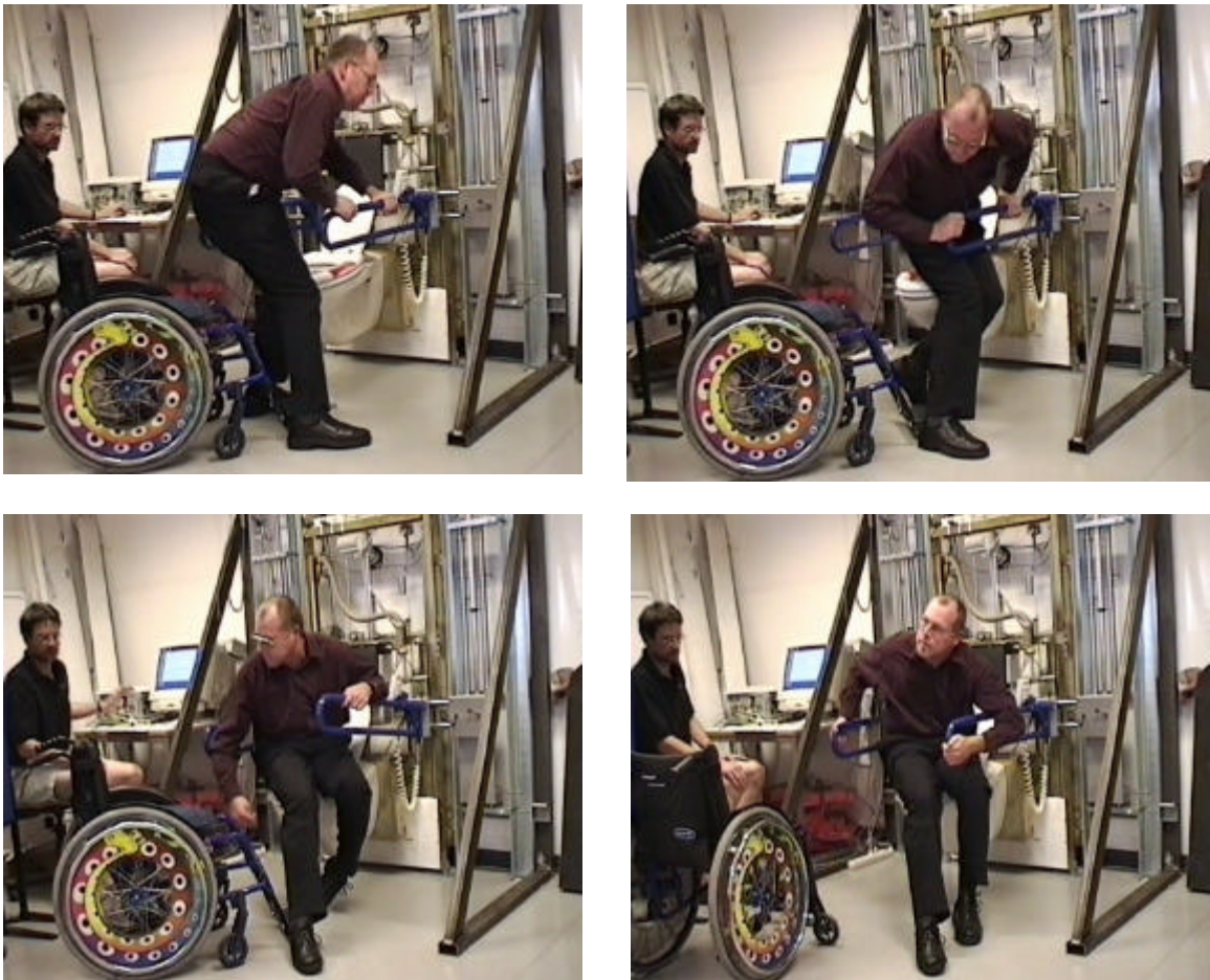
Fig. 2: FRR Test Site in Vienna during one of the first user tests carried out in September 2002. A person in a wheelchair is autonomously transferring from the wheelchair to the toilet. In the background a technician is working in front of the PC which controls actuators and reads sensor data of the toilet assembly, a significantly modified Hungarian product from Clean Solution Kft [19].
