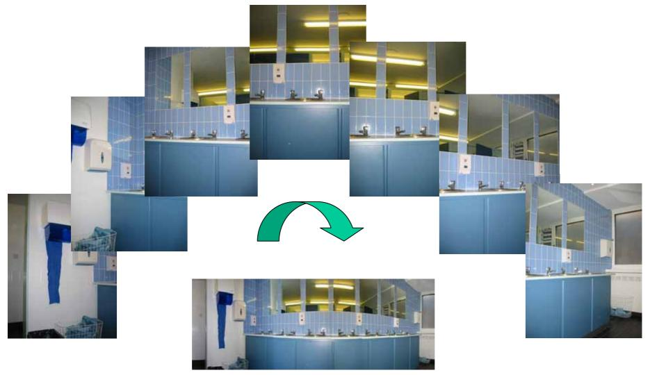
360's created by 'stitching' together a sequence of digital photographs taken by a camera on a tripod in the centre of the scene
