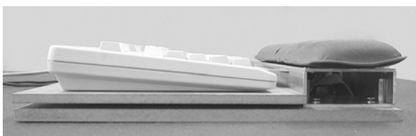
Figure 3: Standard keyboard placed on an experimental pressure sensitive ground plate
