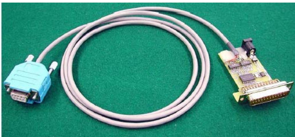
Fig. 5: UST Hardware with removed cover
