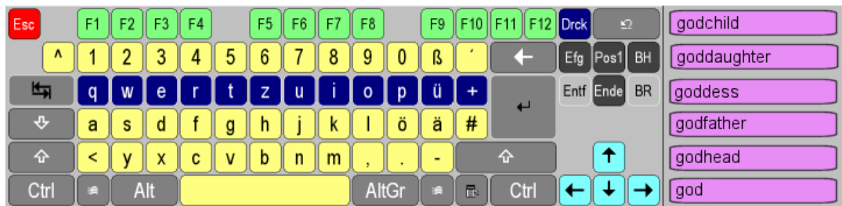
Fig. 2 Example for an OSK with prediction list (used e.g. for a first idea collection)
