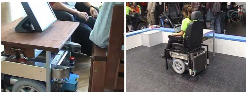
Fig. 20: ICT automatically brought on demand to user sitting in simple chair and Rehacare demonstration
