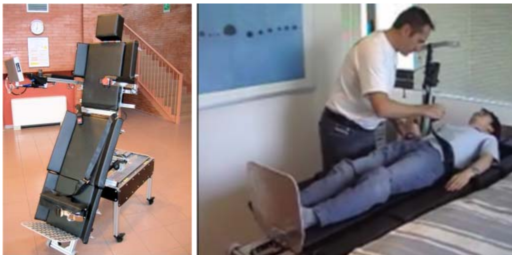
Fig. 16: Movement prototype Multi Functional Chair (MFC) and transfer of user from MFC to bed
