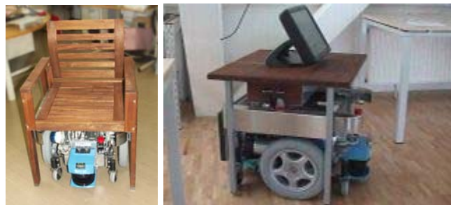
Fig. 5: First prototypes of platform docked to (simple) Chair and ICT
