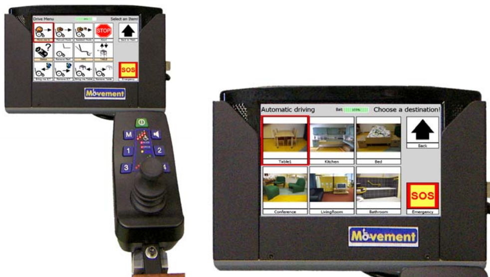
Fig. 11: User interface as seen from chair and exemplary menu for automatic driving
