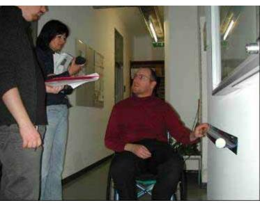
A new type of a "wall mounted body support bar" was developed intending to provide some type of guidance for the fragile users. It failed the user tests as a power grip around the bar was not fully possible (right side of right picture shows the improved well working version tested in the end of
