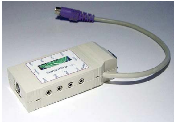
Fig. 3. Interface box for pressure sensitive single switches
